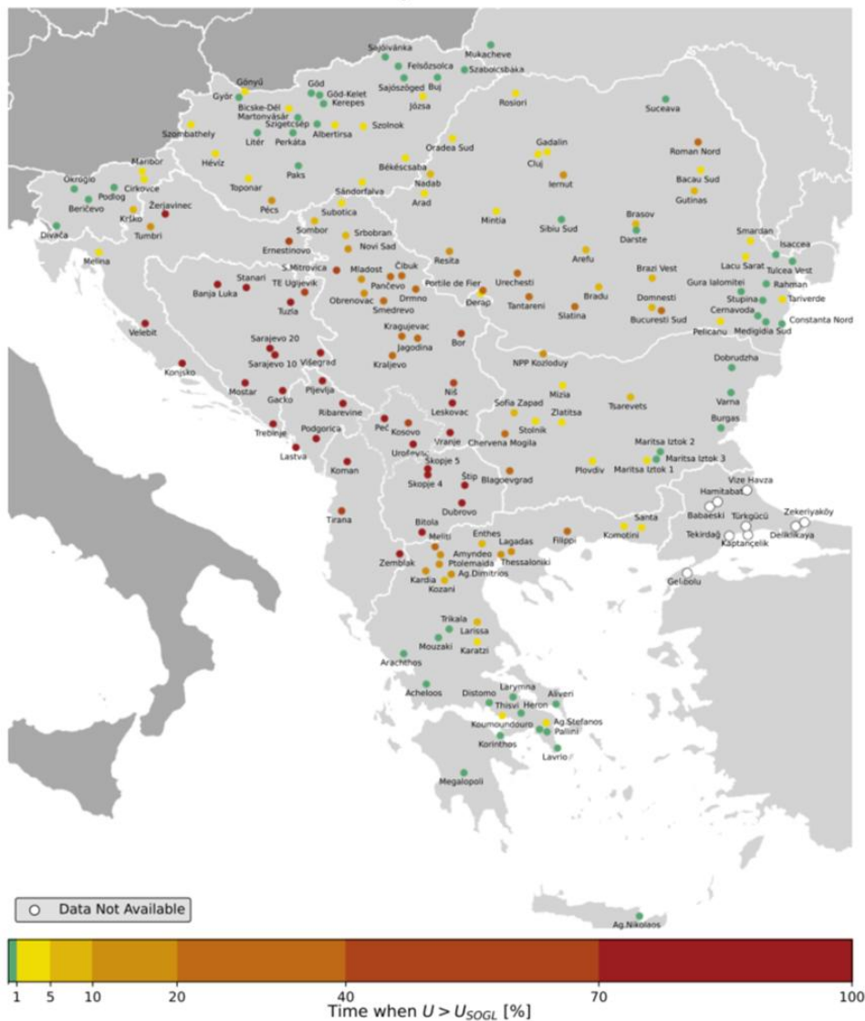
400 kV SS voltages exceeding SOGL limit 420 kV in Southeast Region for year 2025
